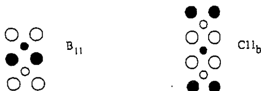
Figure 1. Structures B11 and C11 b . The structures are projected on a (001) plane. The large circles correspond to sites on (00 n ) planes, and the small circles to sites in (00 n + \frac{1}{2} ) planes ( n integer).
